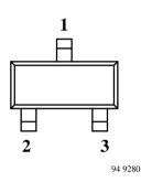
BF799 Marking: G2 Plastic case (SOT 23) 1= Collector; 2= Base; 3= Emitter
